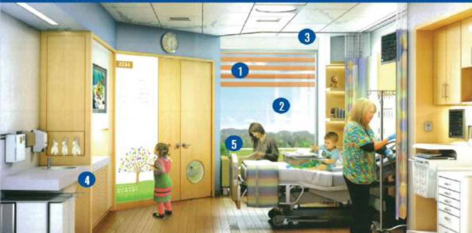
PHOTO 1 Patient room. 1) BMS-activated automatic shading; 2) natural lighting; 3) radiant panels; 4) integrated DV; 5) window planters fed from a recycled water drip irrigation system.
